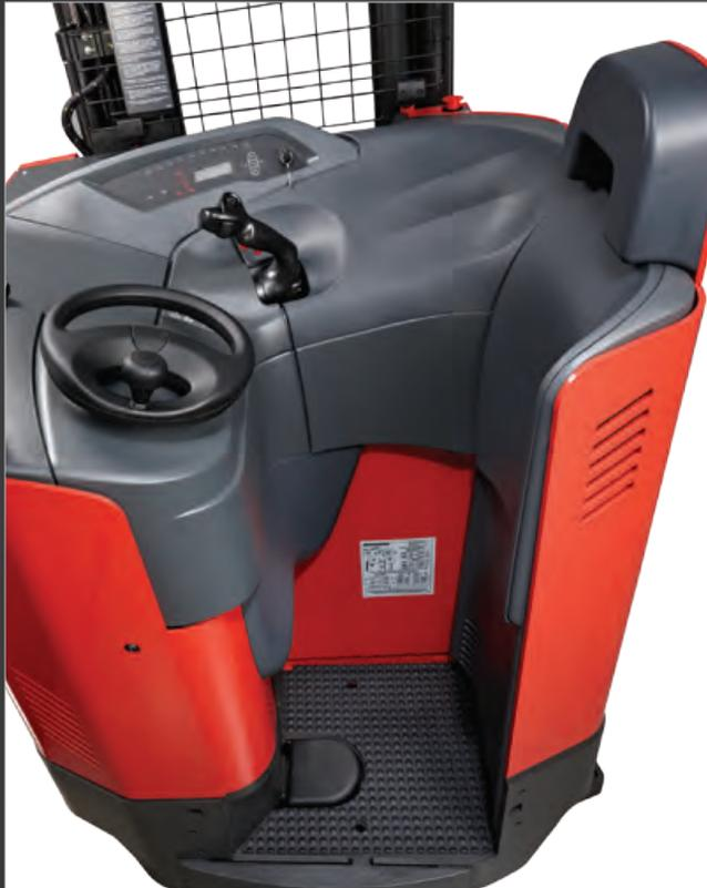
Compartment designed to allow operators to vary positions through the shift. Three elbow/forearm rest positions provide a comfortable, ergonomic workstation.
