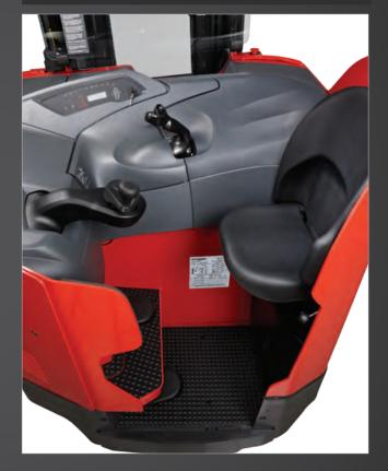
Compartment designed with a cushioned suspension ride seat that flips up for standing operation, and has an adjustable steer tiller.
