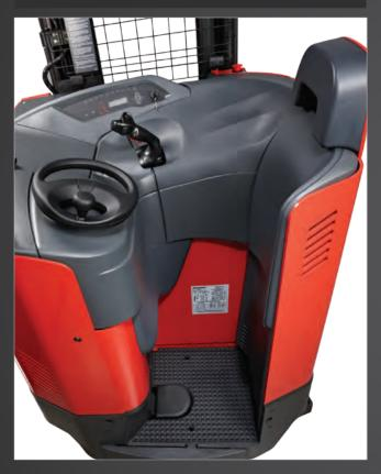
Compartment designed to allow operators to vary positions through the shift. Three elbow/forearm rest positions provide a comfortable, ergonomic workstation.
