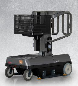
With a compact design, easy maneuverability, electric lift mechanism and driving capabilities, the Sprint 2.0 offers a more efficient and productive alterative to bulky rolling ladders in a variety of environments and applications.
