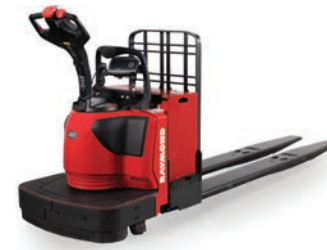
8410 END RIDER PALLET TRUCK + 6000 lb. capacity, 8000 lb. capacity
