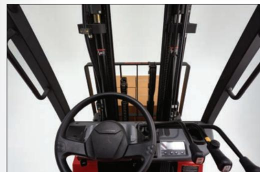
Open view mast provides the best line of sight for the task at hand.
