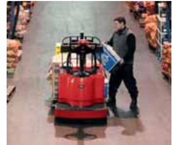
Raymond's CoastPro™ system can be activated with only one hand, for faster order picking.
