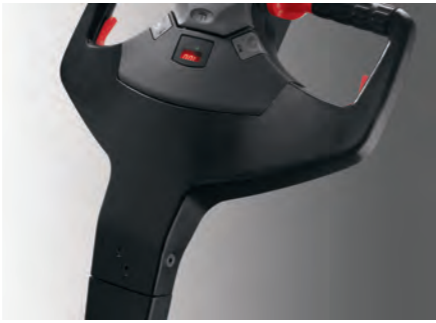
Easy-to-remove handle simplifies service – just remove four screws.
