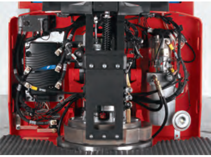
All components are conveniently and logically arranged for faster maintenance: electronics on the left, hydraulics on the right.
