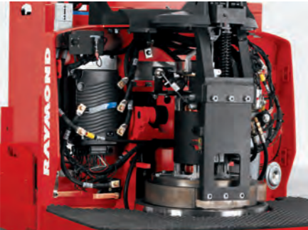
New end bell bracket allows easier access to the brakes.
