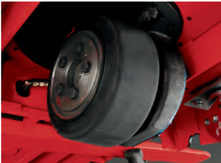
Drive tire is more accessible and easy to change – just remove five bolts. It's like changing a car tire. There is no need to disassemble the transmission.
