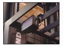
Certain load handling situations require more light than that provided by existing warehouse lighting systems. Work area lights are normally mounted in pairs, providing light to illuminate dimly-lit storage areas. As a consequence, work lights may thereby reduce operator eyestrain and increase productivity. The lights are individually adjustable by the operator to the application requirements.
