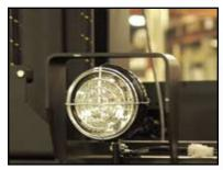
In certain environments of use, an operator must travel from a well lit area to an area of low light. In such environments, travel lights may be of assistance to an operator by illuminating the path of travel. Lights also assist visibility when loading and unloading over the road trucks. Operation travel lights are available singly or in pairs and are automatically activated to illuminate the aisle when the operator activates travel control.
