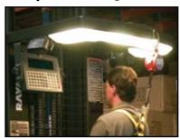
The quality of warehouse lighting may vary throughout the warehouse. In this situation, an operator may have difficulty reading paperwork. Auxiliary lighting may be mounted across the overhead guard to ensure adequate lighting for the operator.
